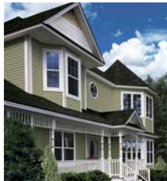
Siding: MainStreet Double 4" Clapboard in Cypress. Accents: Cedar Impressions Half-Round Shingles in Colonial White and Natural Clay. Trim: Vinyl Carpentry® & Restoration Millwork®.
